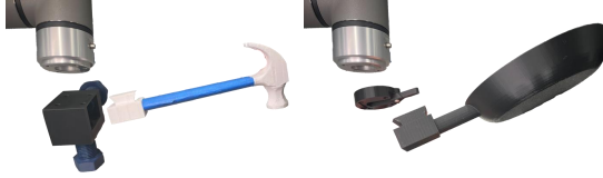
Fig. 13: Fast Tool Changer . Two designs are shown: the left accommodates general tools with a screw mechanism, and the right clips onto tools with specific mounting shapes.
