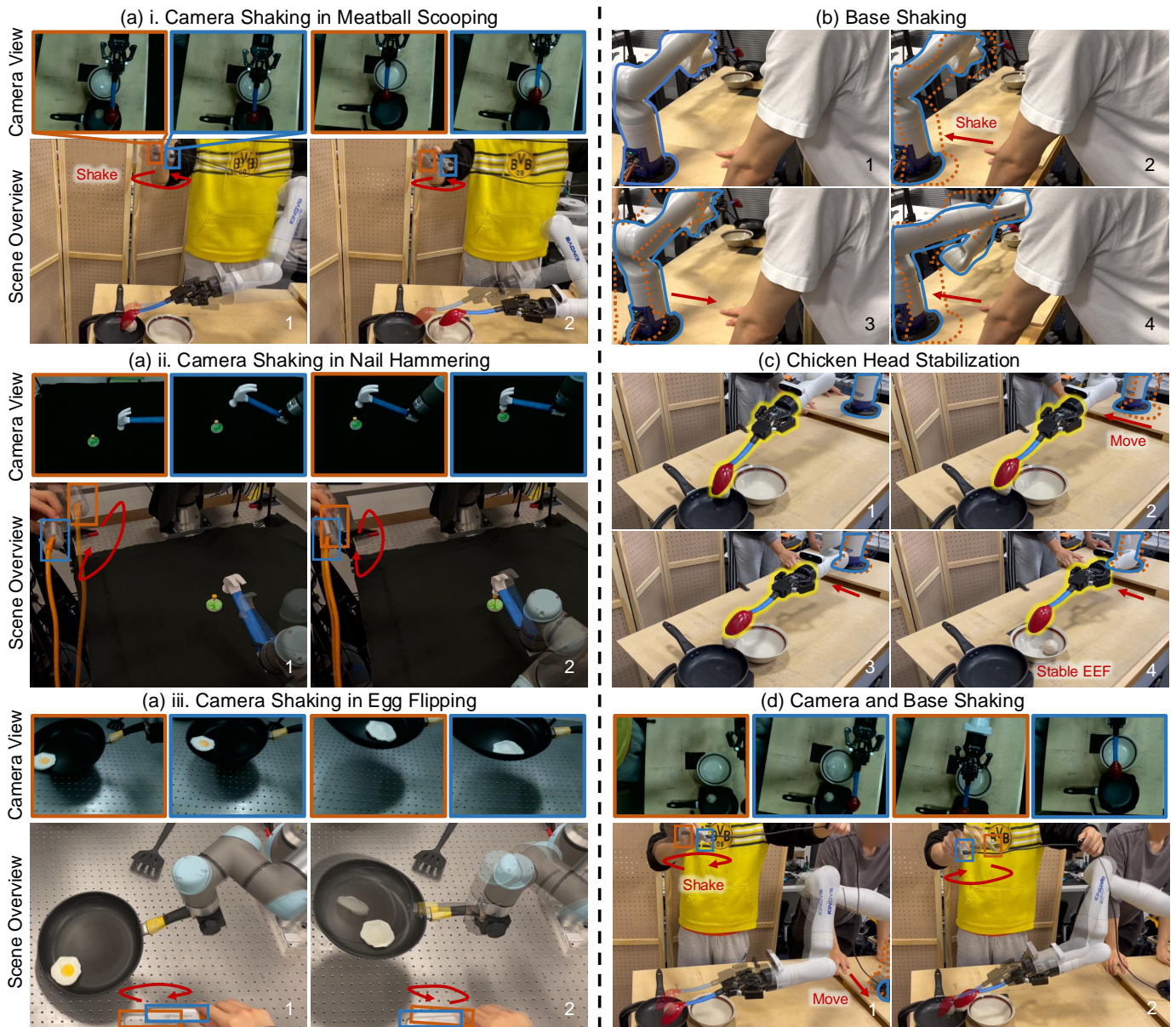
Fig. 8: Robustness to Camera and Base Movement. (a) Camera Pose Robustness: The policy demonstrated the ability to handle camera shaking across three tasks—meatball scooping, nail hammering, and pan flipping. The first row shows the camera view, while the second row provides a scene overview with the shaking motion. (b) Robot Base Robustness: The policy successfully compensated for base shaking, even when the shaking frequency exceeded the robot’s control frequency. (c) Chicken Head Stabilization: At lower base movement frequencies, the end effector displayed a stabilization effect similar to a chicken’s steady head. (d) Combined Robustness: The policy maintained task performance under simultaneous camera and base shaking.
